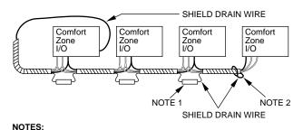
1. Use butt splices, or solder, for shield connections. Then tape up shield.
